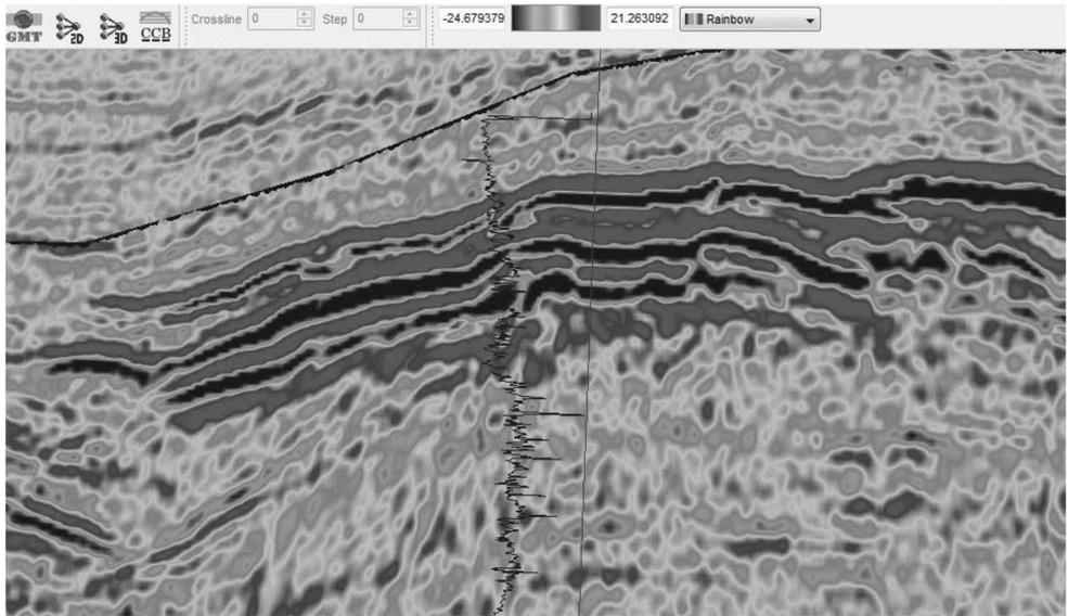
Fig. 10. 1569 line colored inversion profile of LW3-1
